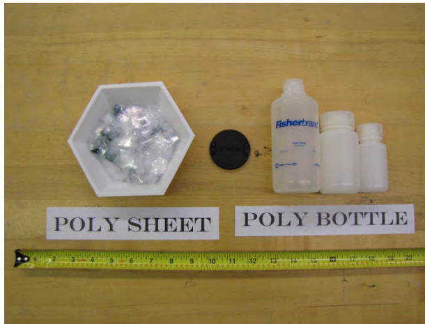
Figure 8. Poly sheet and poly bottle constituent materials.
