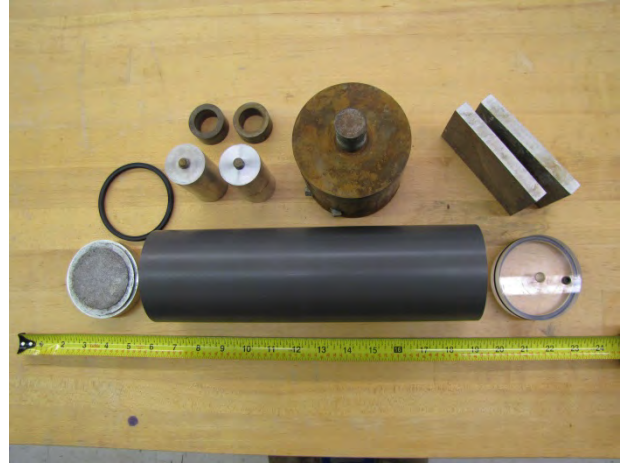
Figure 13. Aluminum jacket and associated hardware for sample assembly and load-cell introduction.
